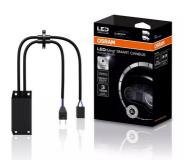
Some vehicles report a malfunction in the exterior lighting when LED lamps are used. With the new OSRAM LEDriving Smart Canbus LEDSCT10, potential error messages in the on-board system are avoided. These error messages can occur when converting to LED lamps as these have a lower current consumption than e.g. halogen lamps and thus activate the vehicle's existing error detection mechanism.
